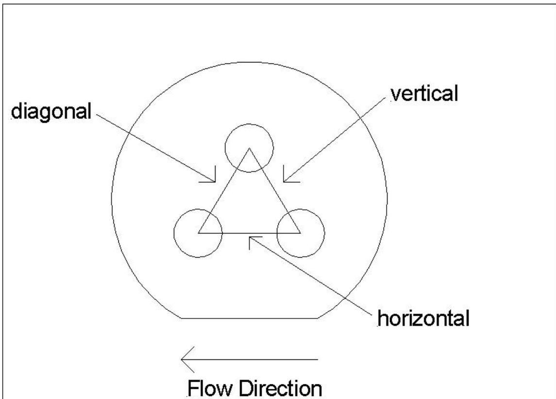
**Figure 1. Schematic illustration of the triangular array of transducers incorporated in each ASFM transmitting or receiving unit. The included labeling denotes the terminology used in the text to identify each of the 3 different transducer pairings (horizontal, diagonal and vertical) as defined relative to the indicated flow direction.**
