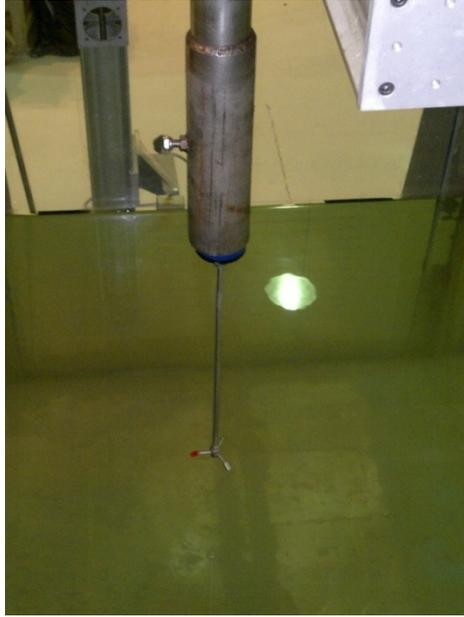
Fig. 5. Acoustic Doppler probe.
