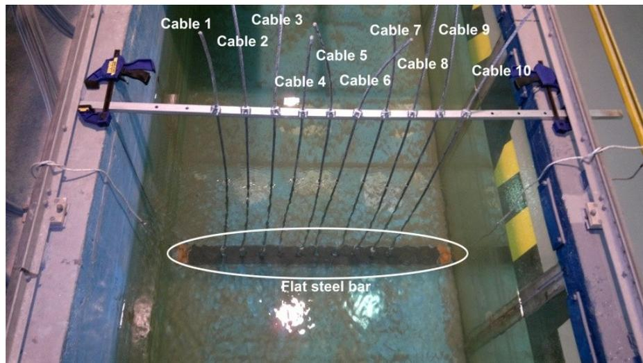
Fig. 4. Cable curtain upstream of the scintillation frame.
