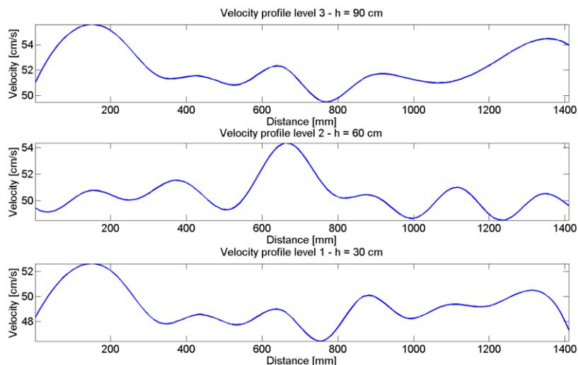
Fig. 6. Horizontal profiles provided from the Doppler probe.
