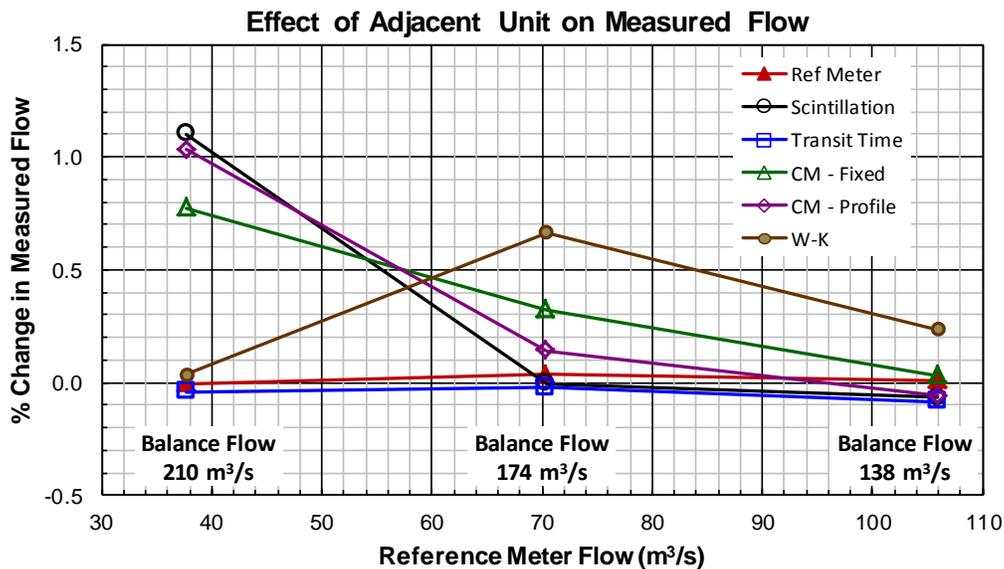
**Figure 14. Effect of Adjacent Unit Operation**
