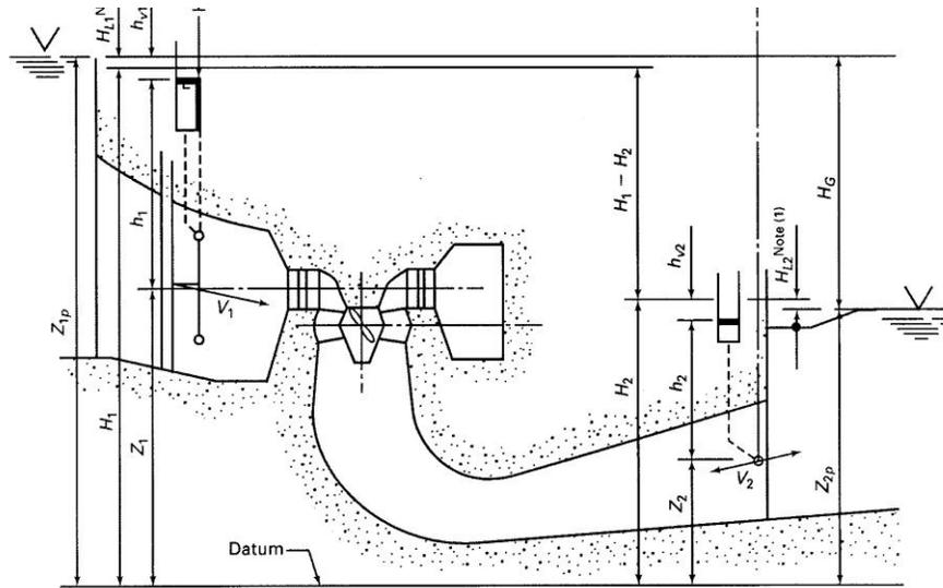
**Figure 1. Typical Kaplan unit short, converging intake**
