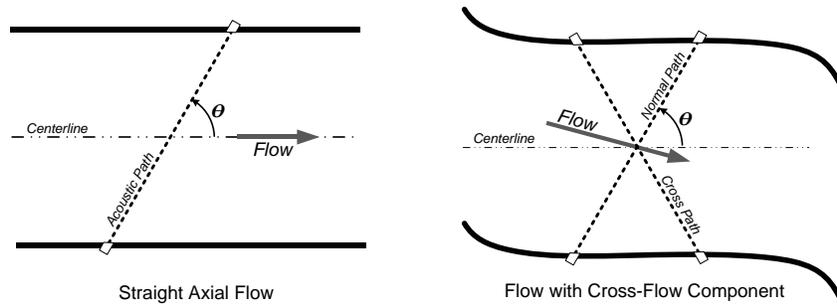
**Figure 2. Acoustic Transit Time Flowmeter Principle of Operation**
