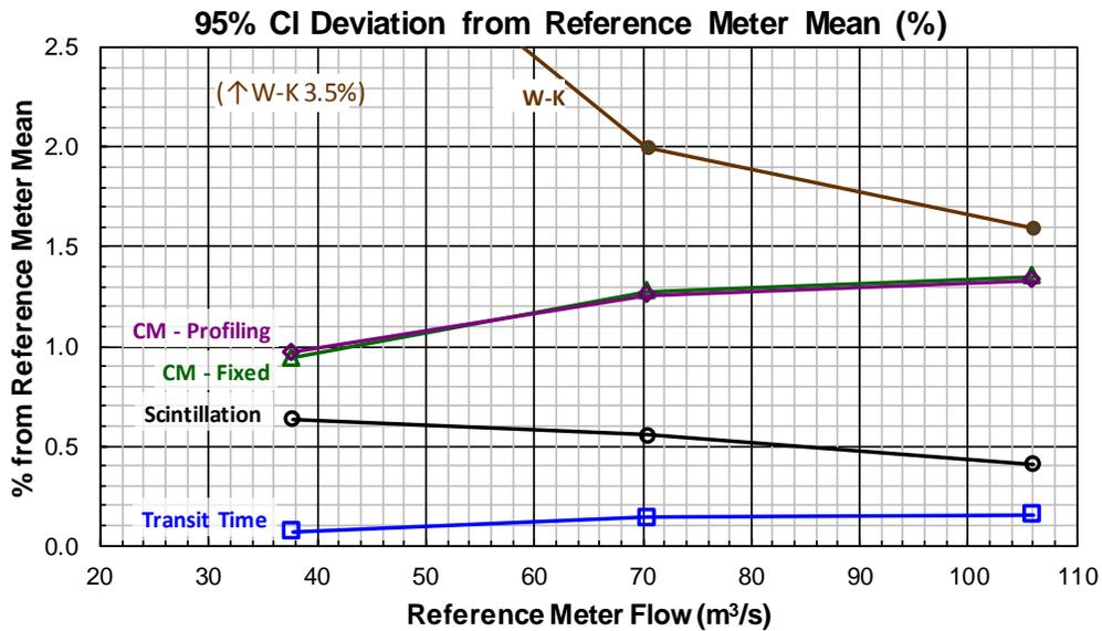
Figure 13. Deviations from the Reference Meter at 95% Confidence
