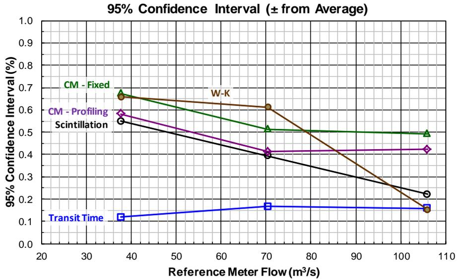
Figure 12. Variability of Test Data for Each Method
