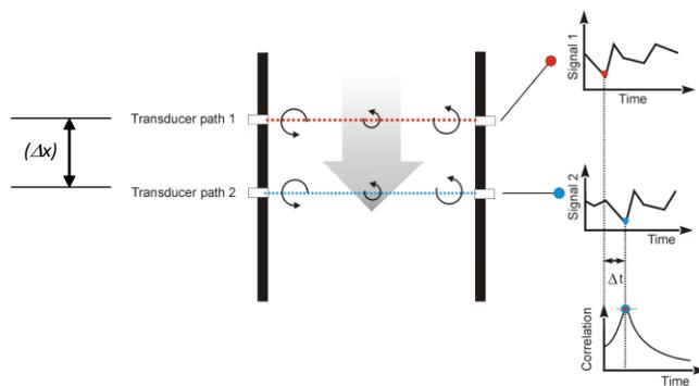
**Figure 3. Acoustic Scintillation Flowmeter Principle of Operation**
