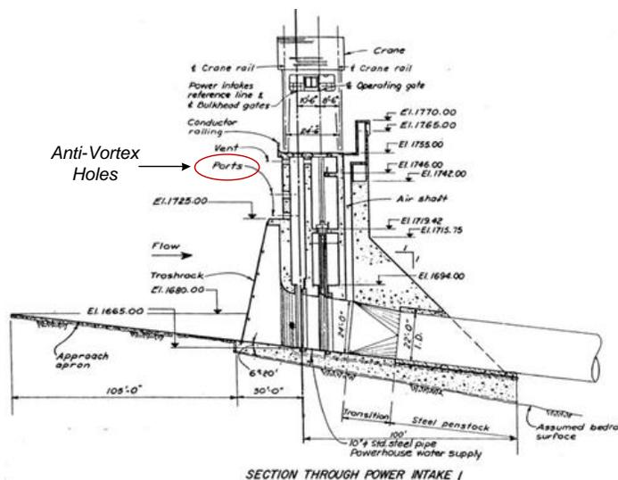
**Figure 4. Unit 1 Intake at Kootenay Canal**
