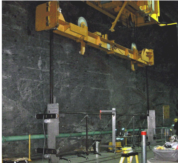
Fig. 7 – Current meter trolley attached to a gantry lifting beam
