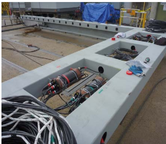
Figure 5: A view of the ASFM equipment mounted on the frame.
